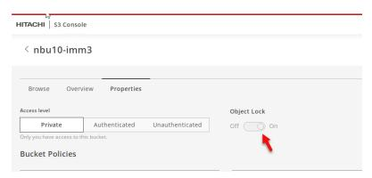
This indicates that Veritas NetBackup can create an object lock bucket on HCP for cloud scale.
