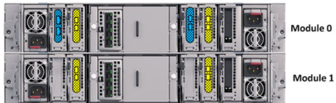
Hitachi Advanced Server DS7040 populated with PCIE cards (Back)
