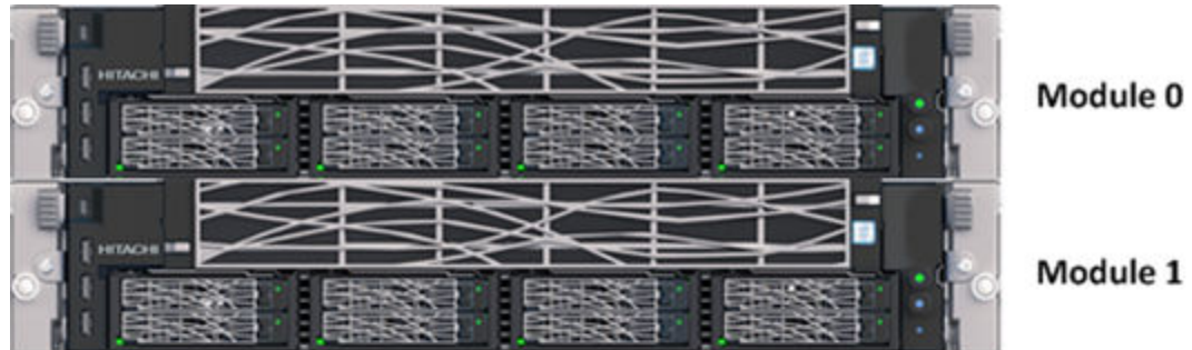
Hitachi Advanced Server DS7040 (Front)
