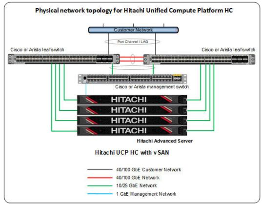
The following diagram represents a standard architecture for the Hitachi Unified Compute Platform HC (with VMware vSAN).
