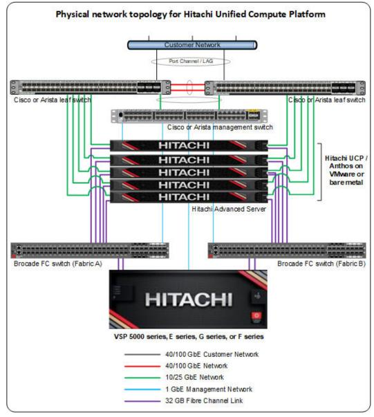
The following diagram represents a standard architecture for the Hitachi Unified Compute Platform product portfolio that supports both VMware and bare metal deployments.
