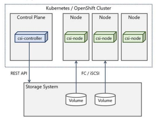
The following diagram illustrates a container environment where Storage Plug-in for Containers is deployed.
