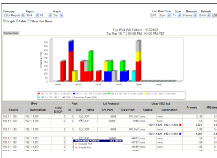
Figure 3. The Brocade Network Advisor Traffic Analyzer feature provides an efficient way to view, retrieve, and report sFlow monitoring data.
